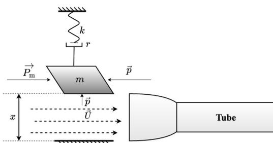
Figure 1. Mass-spring physical model of lip reed.
